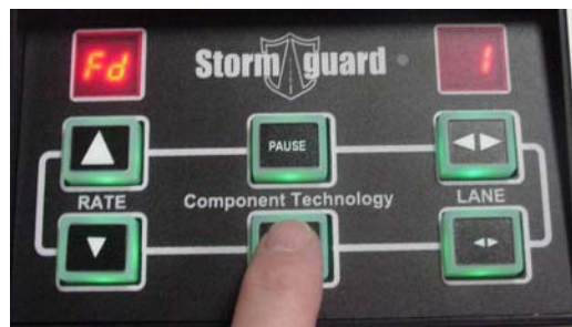
Menu 4 Float Delay Setting
