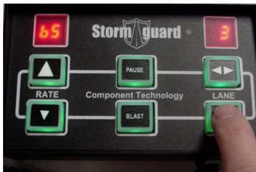
To change menu setting press Lane increase or decrease switch
