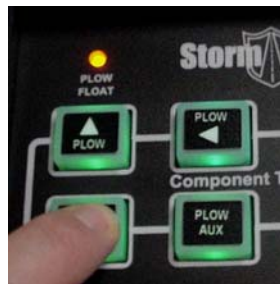
Push and hold Plow Down switch to engage Plow Float
