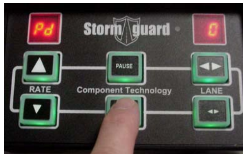
Menu 3 Plow Mode Single or Double acting
