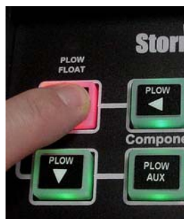
To stop Plow Float push the Plow Up switch
